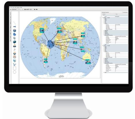
*iTrinegy's NE-ONE Enterprise can simulate "handover" at the IP level and its programmatic control allows extremely rapid LEO network parameter changes*
